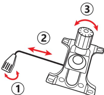
You can change the height of the chair and angle of the seat by the butterfly mechanism.
