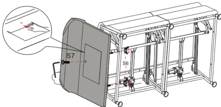
**5. Install the left side frame, screw in the S7 bolt and tighten the S6 wing nuts.
