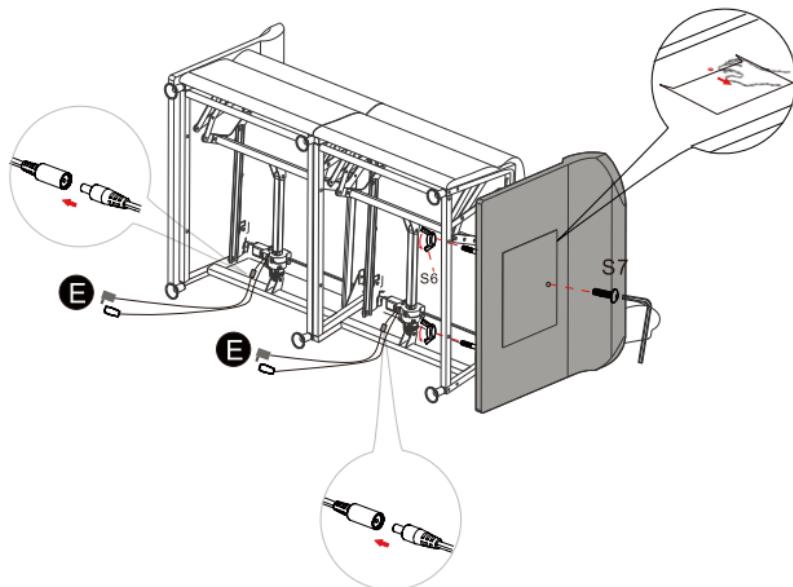
**6. Connect the power supplies to the outlets. Use the right remote control to unfold the right half and the left remote control to unfold the left half**
